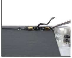
• Use a fine-tip probe or pick to gently peel the dual microphone assembly away from the case.
