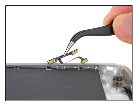
Remove the dual microphone assembly.
