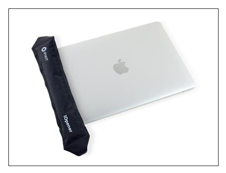
Prepare an iOpener and apply heat to the upper case directly behind the microphone assembly.
