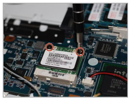
Using the Phillips #00 screwdriver, unscrew the two 4.9 mm screws that connect the WiFi card to the motherboard.
