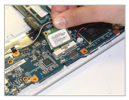
• Using your fingers, lightly grasp the wifi card and firmly pull up and out on the card in order to release the wifi card from its socket.
