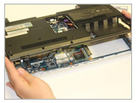
After proper removal of all necessary screws, gently lift up on the back case to remove it.
