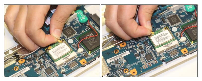
Using your fingers, grasp the white and black wires connected to the wifi card. Pull up on these
