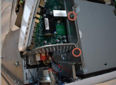
The drive is held in by two phillips #2 screws on each side. Remove these.
