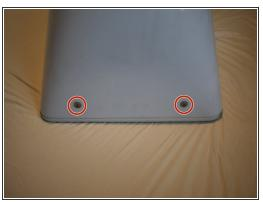
Remove two 2.5mm hex screws from each of the other sides of the computer.
