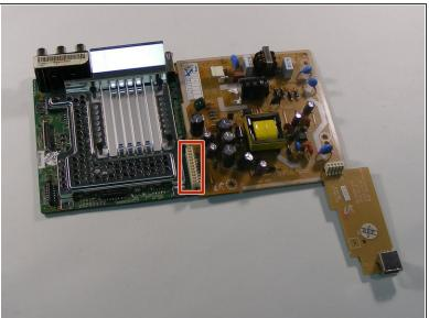
Labeled with a red rectangle is the location where they are connected. Grab the motherboard in one hand and the power supply in the other, and pull the motherboard up and push the power supply down. The motherboard and power supply should then disconnect.
