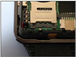
Next we need to remove the 4 screws in the corners, These can be removed with a 00 head
