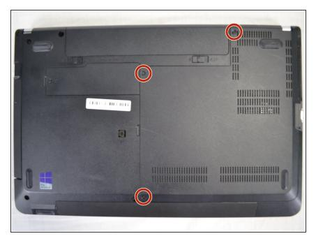
Remove the three 1.2mm Phillips #00 screws from the bottom panel.
