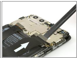
• Use a spudger to disconnect the interconnect, the battery and the display flex cable.
