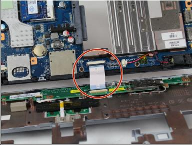
Open the top carefully without disconnecting the two parts.
