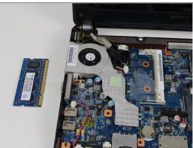
Carefully press the sides near the right edge of the part and remove it from it's base.
