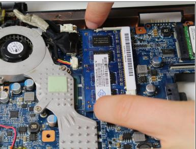
Using your fingers, pry apart the two side metal pieces that hold the part in place as shown on the picture.
