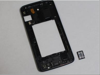
Use the tweezers to lift the loudspeaker out of place.
