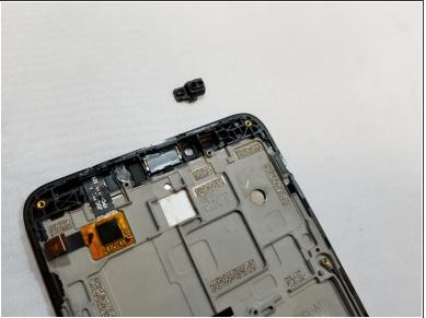
• Remove the camera's rubber seal by lifting it out with a pair of tweezers; it should come out easily.
