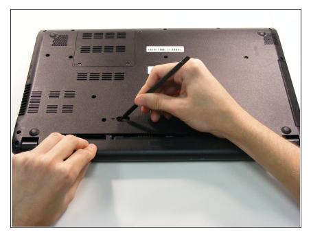
Use the pointed end of the spudger to slide the battery lock until the battery pops loose.
