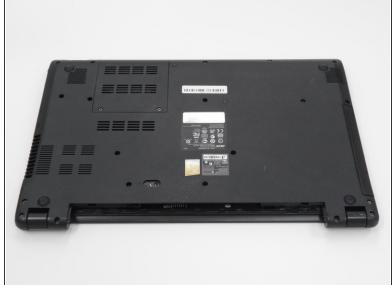
Slide the battery out of the battery slot.
