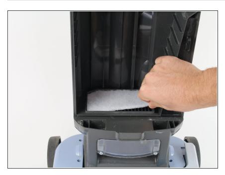
Remove the old inlet filter from the vacuum body and replace with the new filter.
