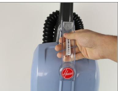
Remove the frame of the vacuum by pinching the tab down and pulling the frame away from the vacuum body.
