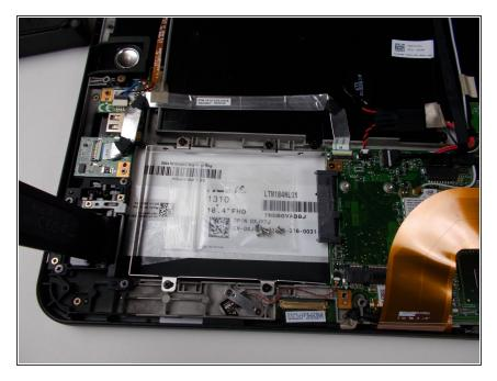
I'm installing an mSATA SSD in mine, so I put these screws in a small plastic bag, taped them in the empty space the HDD occupied, and screwed the caddy back into place.
