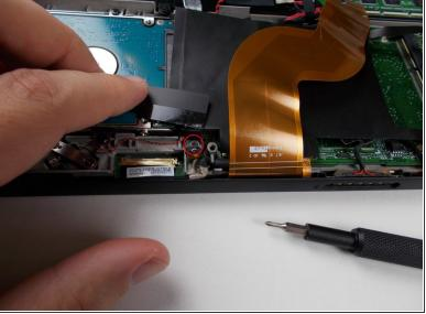
There are two screws that hold this plastic sheet down because it's also a grounded shield. Use the #0 screwdriver to unscrew the screws shown in these photos.
