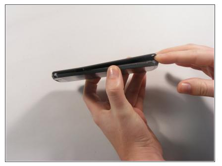
Insert fingernail into the slot on the back left side of the phone and pry open.
