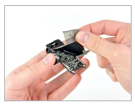
Continue peeling the EMI tape off the bottom of the AirPort/Bluetooth bracket and remove it from the assembly.
