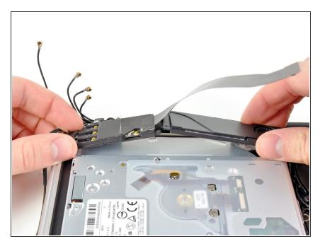
Pull the AirPort/Bluetooth assembly and the Subwoofer upward near the center of the side of the optical drive until they clear each other.
