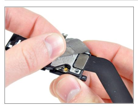
Peel back the piece of EMI tape covering the AirPort/Bluetooth cable connector.
