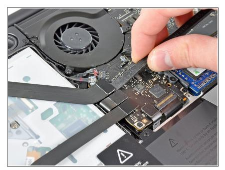
Use the flat end of a spudger to pry the AirPort/Bluetooth ribbon cable connector up from its socket on the logic board.
