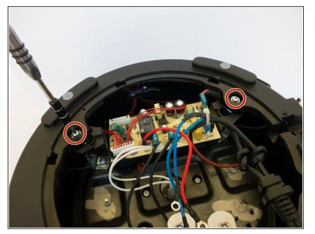
Use a Phillips head #2 screwdriver to remove both 15mm screws from either side of the circuit board, indicated in the picture.
