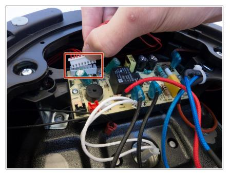
Wiggle the wide white component until it is removed from the circuit board.
