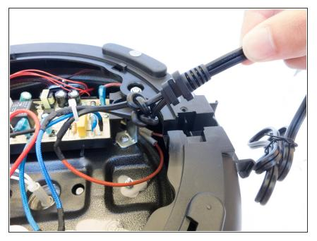
• Remove the power cord from the slot it is inserted in.
