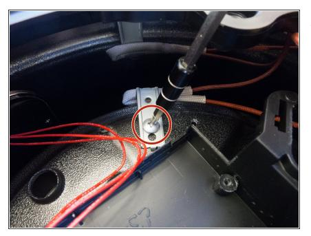
Use a Phillips head #2 screwdriver to remove the 6mm screw behind and to the right of the circuit board tray.
