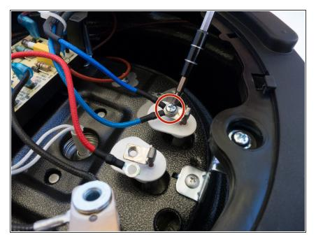
Use a Phillips head #2 screwdriver to remove the 8mm screw and it's washer from the blue wire.
