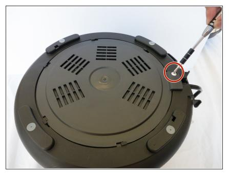
• Use a Phillips head #2 screwdriver to remove the 6mm screw.
