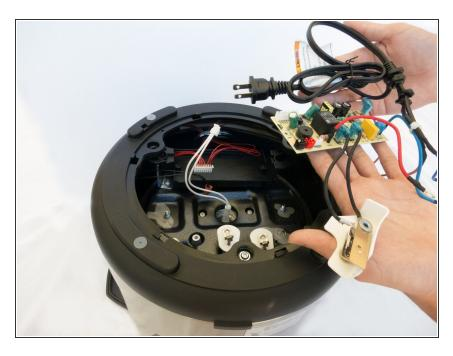
• Remove and replace the circuit board.
