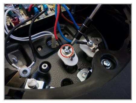
Use a Phillips head #2 screwdriver to remove the 8mm screw and it's washer from the red wire.
