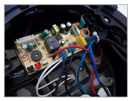
Use a J1 head screwdriver to remove the 8mm screws from both sides of the circuit board.
