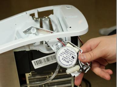
Lift the Water Pump out of the way
