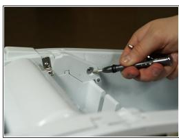
Remove the 4 screws holding the Ice Tray from the top.
