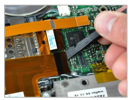
Use the flat end of a spudger to pry the hard drive ribbon cable connector up off the logic board.
