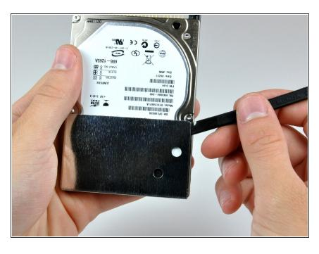
Use the flat end of a spudger to separate the adhesive holding the hard drive shield on the hard drive.
