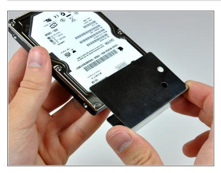
Pull the hard drive shield off the hard drive.
