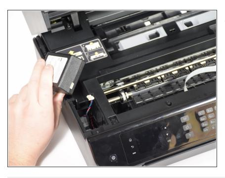
Remove final cable from power supply.
