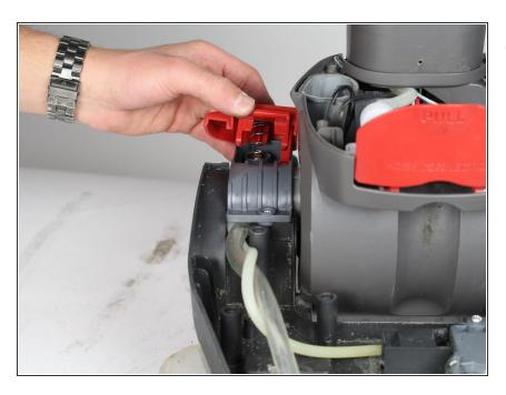
Remove the "On/Off" cap by pulling it upwards with caution.
