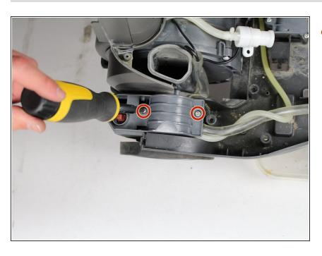
Use a long #2 Philips head to remove the two screws from the arched grey piece.
