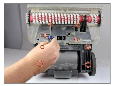
Use a long #2 Philips head to remove the 8 numbered screws on the bottom of the cleaner (They will also be indicated on the bottom of the vacuum).
