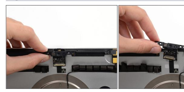
• Lift and remove the camera assembly from the iMac.
