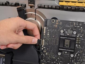
Pull the camera cable straight away from its connector on the logic board.
