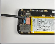
• Use flat edge of the spudger to pry up the two blue connectors near the top of the device.
