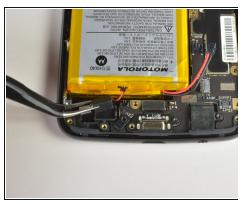
Using a pair of tweezers disconnect the vibrating motors connector near the bottom of the device.
