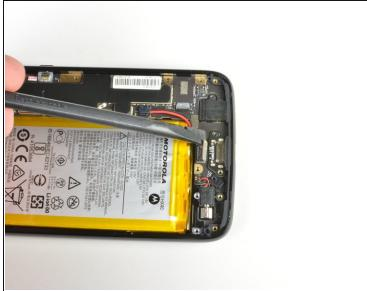
Use flat side of spudger to pry up connector near the bottom of the device.
