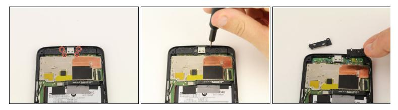
• Unscrew four 1.8mm T4 screws from the speakers and remove from the motherboard.
