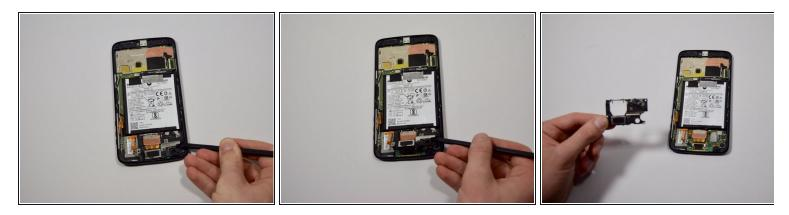
• Use the nylon spudger to lift and remove the speaker from the phone chassis.
