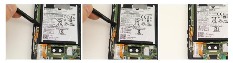
• Using the spudger, lift up the bar on the ZIF connector that joins the ribbon cable to the control buttons.
