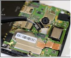
Disconnect the marked connector with a pair of tweezers and remove the camera piece.
