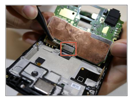
Unplug the back connector from the motherboard using tweezers.
