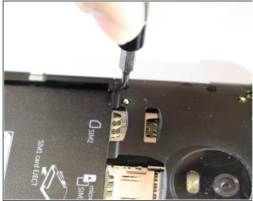
• Remove the eight (8) 4mm screws with a Phillips screwdriver.
