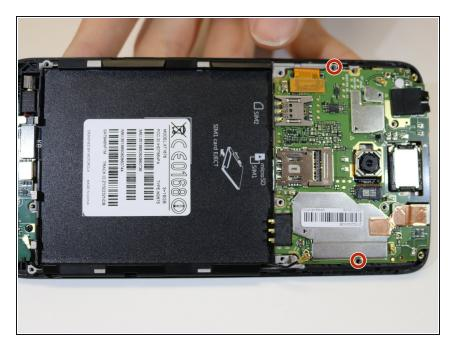
Remove the two 4mm screws shown in the picture using a Phillips #00 screwdriver.
