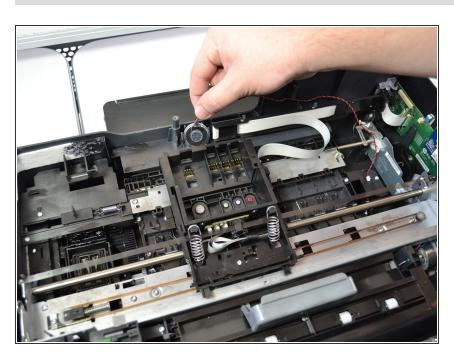
Carefully slide the speaker out of the printer.
