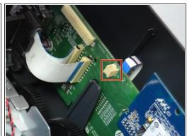
Grab the intertwined red and black wires. Gently pull up and disconnect the wires from the motherboard.
