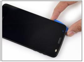
Insert an opening pick as deep as possible under the top left corner of the screen assembly to slice through the left patch of adhesive.
