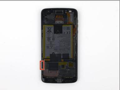
When separating the left side of the screen assembly, take care to not snag the display cable located on the left edge near the bottom of the display.
