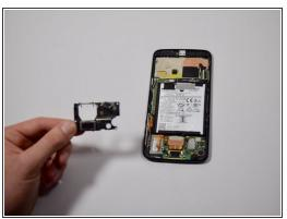
Use the nylon spudger to lift and remove the speaker from the phone chassis.
