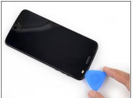
Slide your tool around the top edge of the screen assembly and slice all along it to slice through its adhesive.
