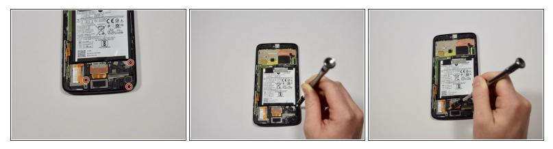
Unscrew the three 1.7mm T4 screws from the speaker.
