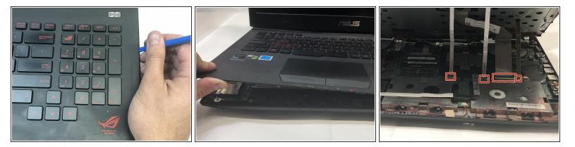
• Use a plastic opening tool to pry the keyboard from the base of the laptop.
