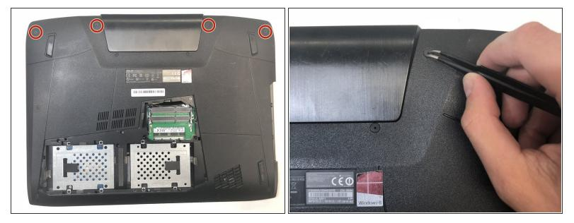
• Use a pair of tweezers to remove the top four rubber stoppers found on the bottom of the laptop.
