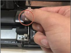
Use a nylon spudger to carefully pry the top back panel off.
