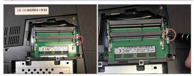
• Use a Phillips 1 Screwdriver to remove the 5 mm screw that is located underneath the back panel.
