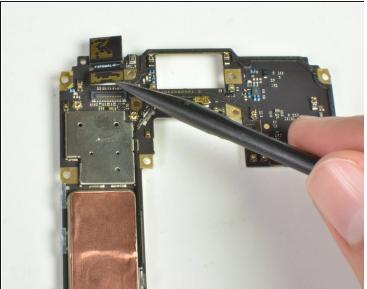
• Now use the flat edge of a spudger to carefully disconnect the camera from the motherboard.
