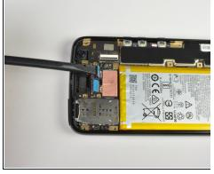
• Use flat edge of the spudger to pry up the two blue connectors near the top of the device.
