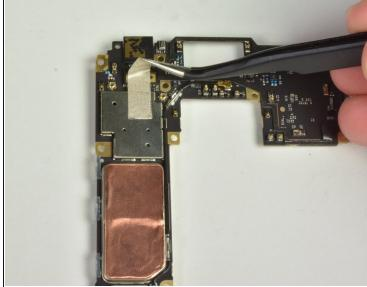
Now carefully peel off the tape on the back of the camera with tweezers.
