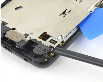
Insert the flat end of a spudger under the lower right edge of the midframe and pry up to release the midframe clip.
