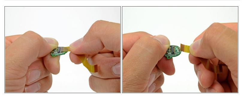
• Pull the camera sensor ribbon cable straight out of its socket on the camera sensor board.
