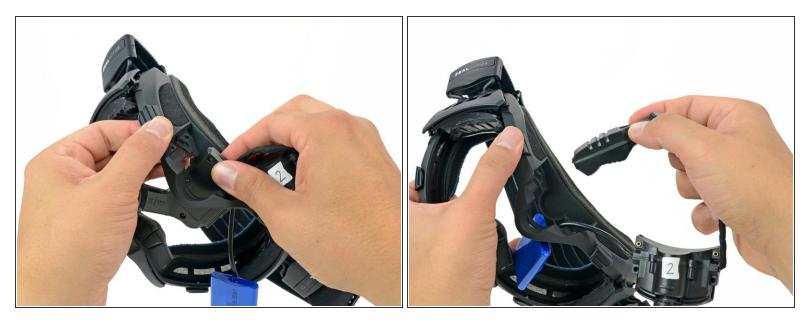
• Remove the viewfinder assembly by pulling it through the opening in the top of the frame.
