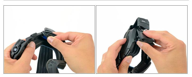
• Once the bottom is free, continue pulling to free the top of the strap mount cover from the frame.
