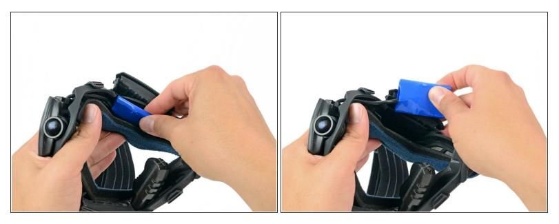
• Pull the battery out of its recess in the frame.
