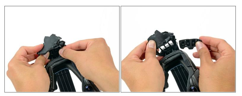
• Hold the strap mount cover away from the frame and remove the keypad.
