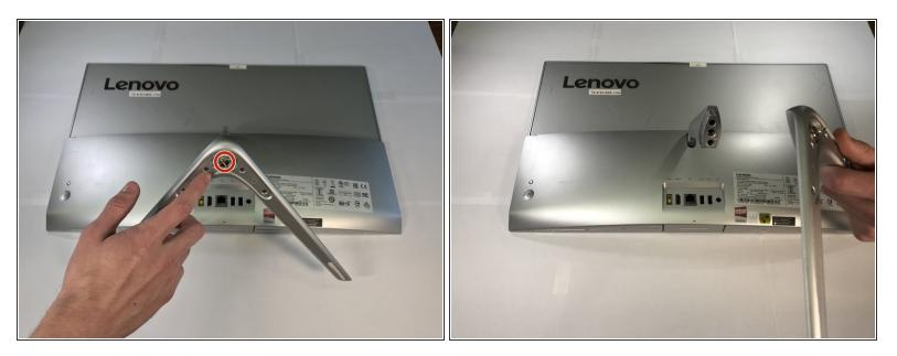
• Remove the monitor stand screw in the bottom of the stand, and remove the stand completely.
