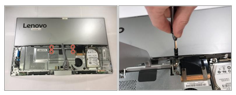
Remove the four screws that secure the arm stand.
