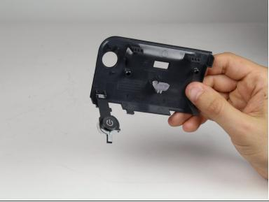
Press on the power button from the front of the panel to release it.
