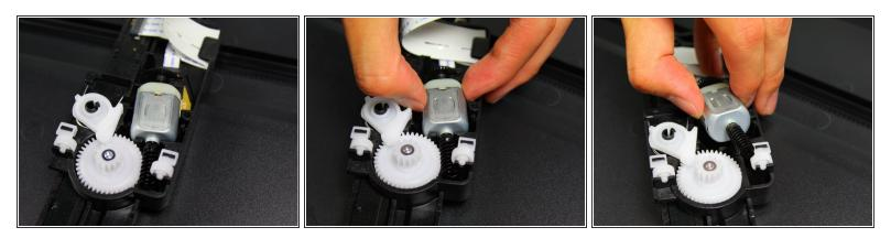
• Remove the motor from its casing by holding the motor on both sides and pulling up.
