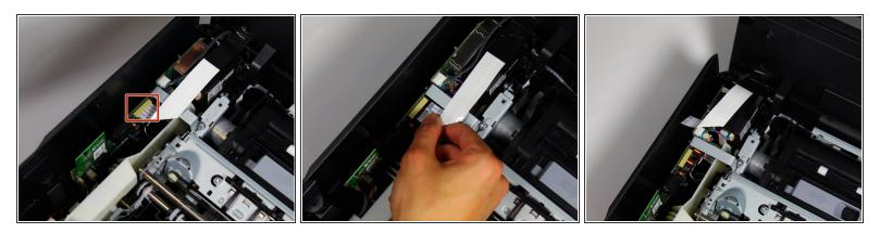
• Remove the connector that binds the cartridge access door to the motherboard by pinching the blue part of the connector with two fingers and pulling it away from the motherboard.
