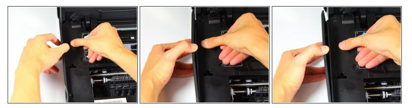
• Detach the left-side panel by applying downward pressure on the internal protective cover with one hand and pulling the left-side cover with the other.
