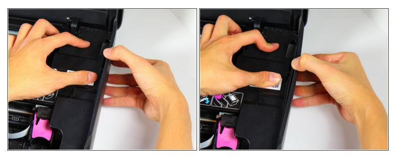
• Detach the right-side panel by applying downward pressure on the internal protective cover with one hand and pulling the right-side cover with the other.
