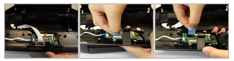
Remove the connector that is attached to the screen's circuit board by pinching the blue part of the connector with two fingers and pulling it away from the circuit board.
