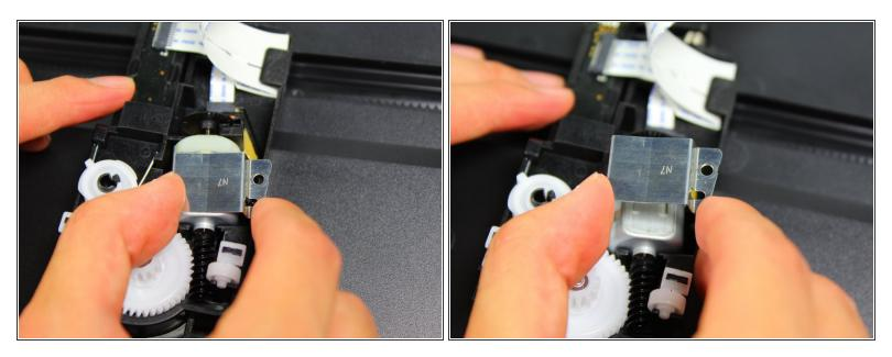
• Remove the metal plate by lifting it away from the motor.
