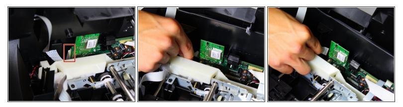
• Remove the connector that binds the internal protective cover to the motherboard by pinching the blue part of the connector with two fingers and pulling it away from the motherboard.
