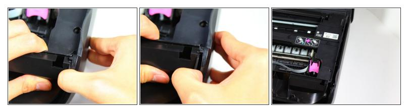
Detach the right-side panel by pulling the right-side cover clip away from the internal protective cover.
