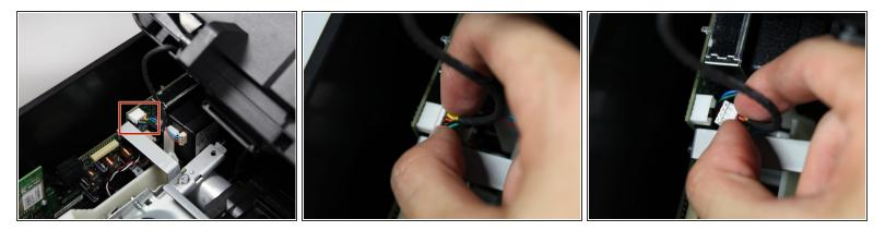
• Remove the cables that connect the cartridge access door to the motherboard by pinching the front of the cable box with two fingers and pulling it away from the motherboard.
