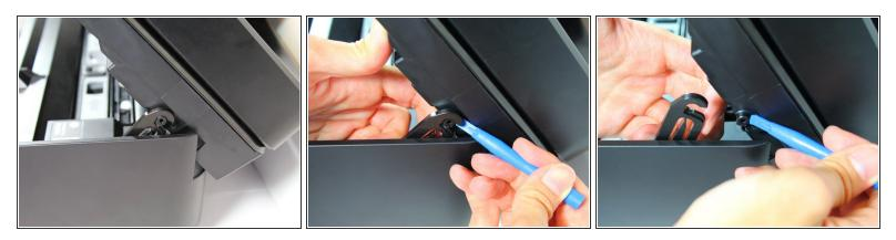
• Unhook the clip supporting the cartridge access door by using a plastic opening tool to get under the clip and using another hand to pull the clip from its hook.
