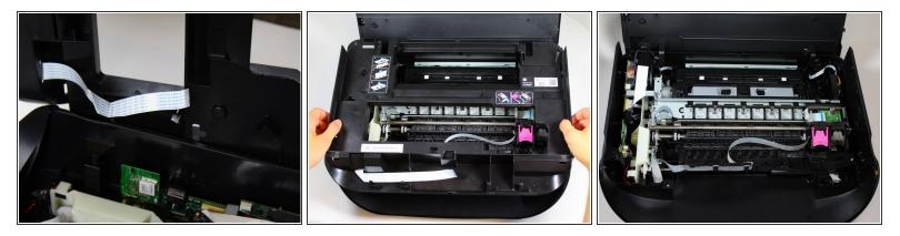
• Remove the protective cover by lifting it away from the printer with both hands.
