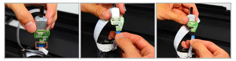
Remove the connector that is attached to the motor by pinching the blue part of the connector with two fingers and pulling it away from the circuit board.
