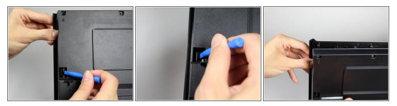
• Use a plastic opening tool to snap off the left-side clip and push the clip outward.
