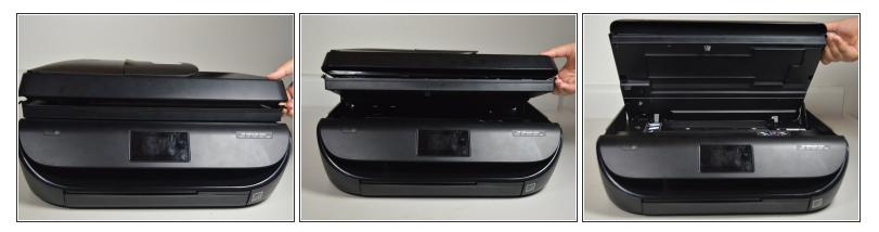
• Open the cartridge access door by placing one hand on the grooves of each side and pulling up.
