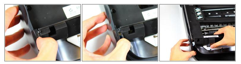
• Pull the left-side cover clip away from the internal protective cover to unhook it from the left-side cover.
