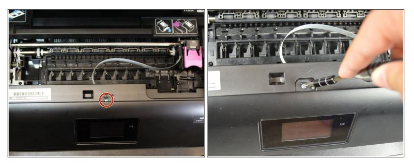
Using the hex screwdriver, remove the 2.0 mm x 14 mm screw that binds the front cover to the printer body by turning the screw counterclockwise.
