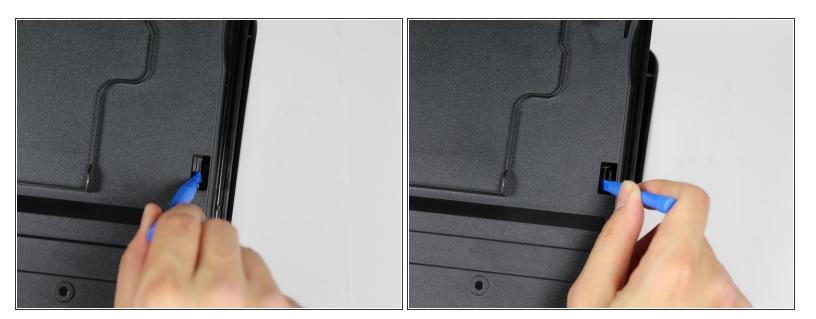
• Use a plastic opening tool to snap off the right-side clip and push the clip outward.
