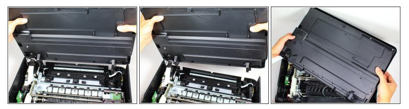
• Flip the cartridge access door with two hands so that the non-glass side of the cartridge access door is on top.
