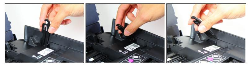
• Release the clip by pushing the clip towards the inside of the printer and pulling the clip out.
