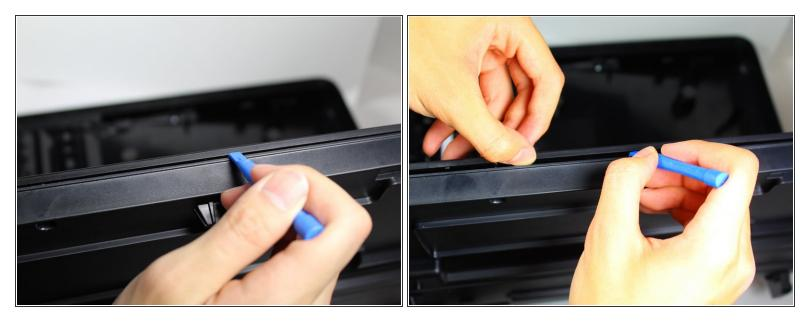
• Wedge the plastic opening tool into the creases on the sides of the cartridge access door to help detach the glass side from the back side of the cartridge access door in the next steps.
