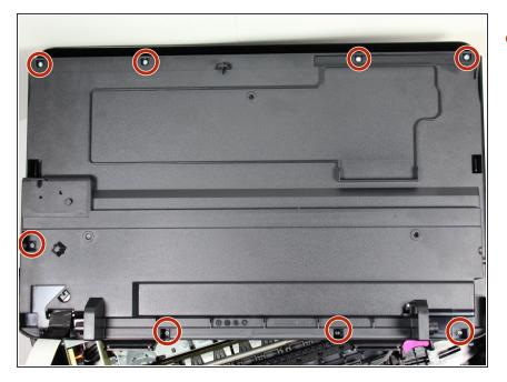
Remove the eight 2.0 mm x 14 mm hex screws on the back of the cartridge access door by using the hex screwdriver and rotating counterclockwise.
