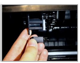
Pull the side cover of the manual one-inch paper-feed roller to the right and remove the paper roller.
