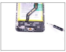
Remove the six 1mm Phillips #0 screws by rotating the screwdriver counter-clockwise.
