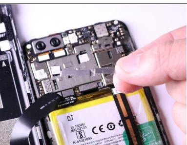
Carefully pop out the metal connector cap with the nylon spudger and remove it by pulling up.
