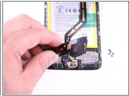
• Remove the loudspeaker by gently pushing the spudger underneath it and prying it out.
