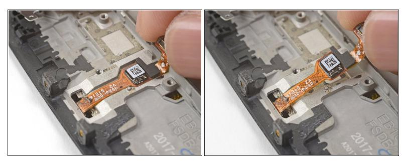
∧ If you are planning to reuse the fingerprint scanner, be extremely careful pulling the flex cable up. It is very delicate and prone to breaking.
