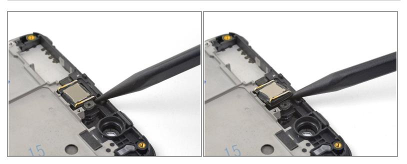
Insert the point of a spudger under the top right corner of the earpiece module and pry up, loosening the module from its recess.
