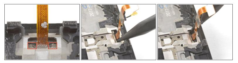
Insert the point of a spudger into the marked areas on either side of the flex cable, and push until the fingerprint scanner is loosened from its recess.
