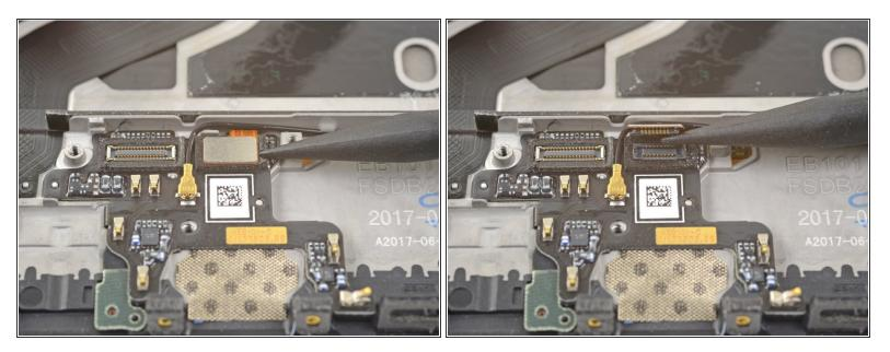
Use the point of a spudger the pry up and disconnect the fingerprint scanner connector from its socket on the daughterboard.
