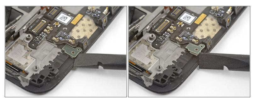
Insert the edge of a flat end of the spudger underneath the microphone board and twist slightly to release the board's adhesive.
