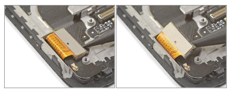
Use the point of a spudger to pry up the display connector from its socket near the bottom left corner of the frame.
