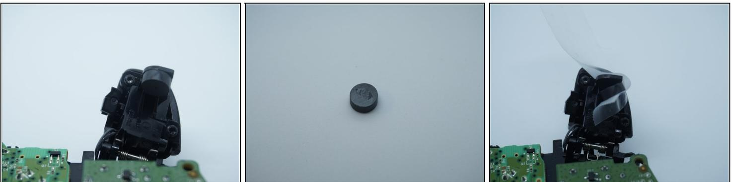
**⚠ Incorrect magnet alignment will result in LT/RT activation without human input.**
