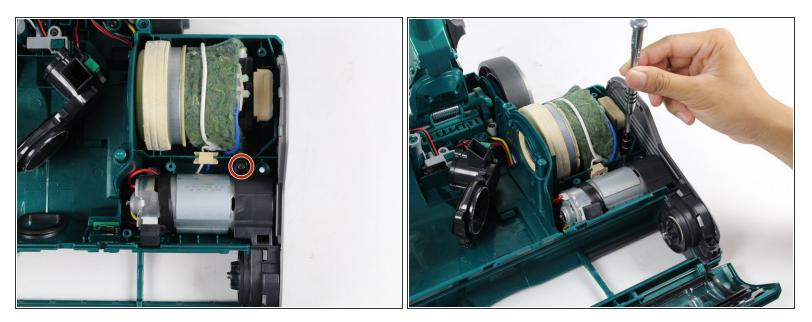
Remove one 14mm screw by rotating counter-clockwise with a T15 Torx screwdriver.
