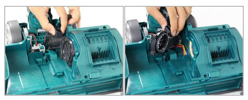
Remove the airpath grille from the side of the motor compartment by pulling out and away from the attached area.
