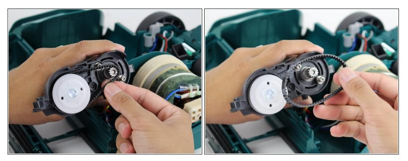
• Remove the belt by pulling the belt away from the axle.
