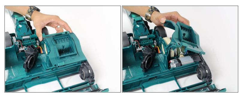
• Remove the motor compartment panel by lifting up and away from the device.
