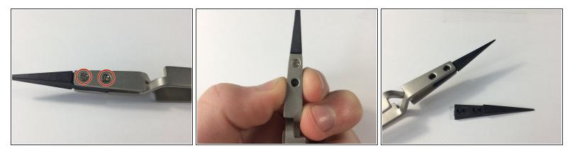
• remove 4 PH0 philips screws, 2 on each side.
