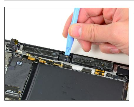
Peel the front camera off the foam adhesive securing it to the rear panel.
