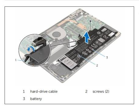
Remove the screws that secure the battery to the palmrest and keyboard assembly.
