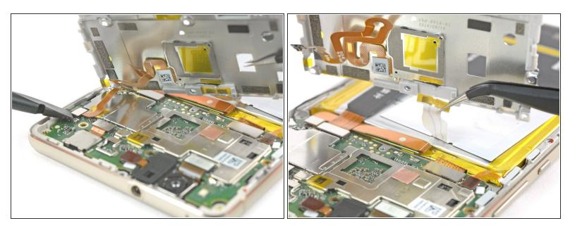
$\bigwedge$  Do not remove the shield plate yet, it is attached by a connector and an adhered cable.
