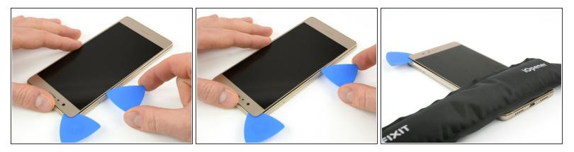
• As long as the adhesive is warm try to continue to separate the display along the side towards the bottom. Re-heat the iOpener if necessary.
