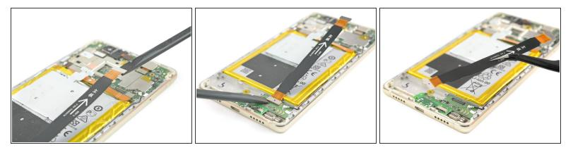
Disconnect the motherboard flex cable on both ends and take it away.
