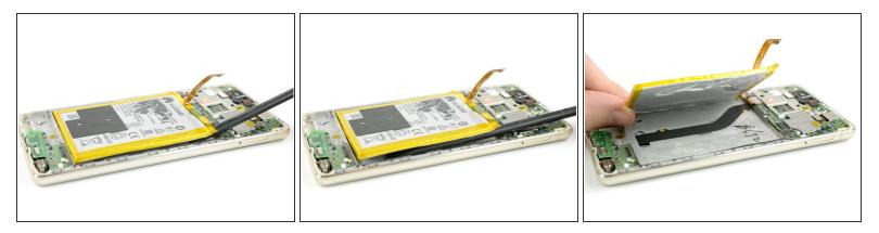
Slide the spudger under the battery at the place shown in the picture and pry it loose slowly.
