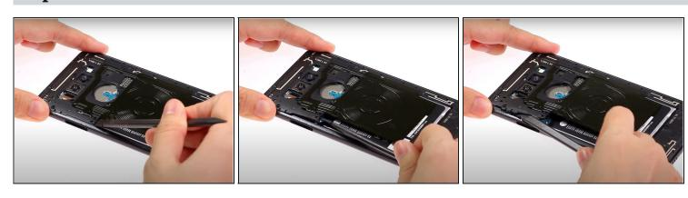
• Using a plastic spudger, pry up the midframe of the phone.
