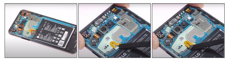
• Use the plastic spudger to pry up the four press-fit connectors on the top portion of the motherboard.
