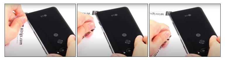
• Continue to slide the cards around the remaining three edges to release the adhesive.
