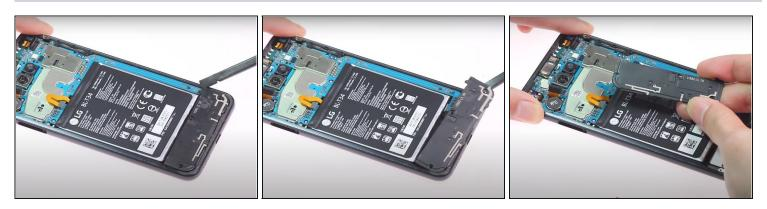
• Pry up the speaker panel with a plastic spudger and remove it from the phone.
