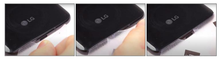
• Insert a second card where you have created an opening with the first card and slide it along the bottom edge of the phone.
