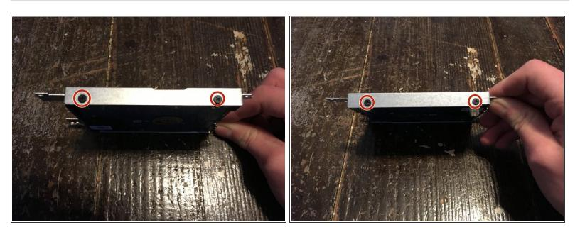
Remove the four Philips #1 screws.
