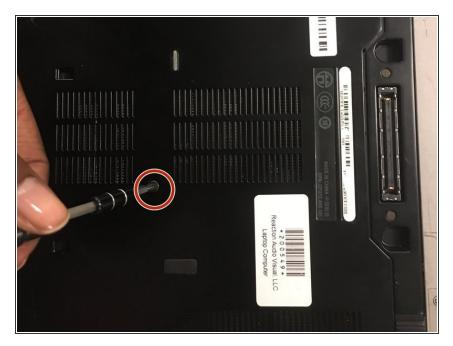
Use a J1 screwdriver to remove the 8mm screw on the bottom cover.
