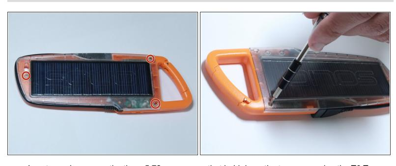
Locate, and unscrew, the three 5.72 mm screws that hold down the top cover using the T6 Torx screwdriver.
