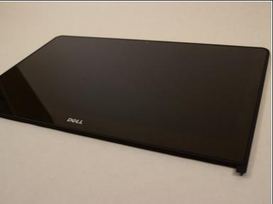
• The display is now fully disconnected, you can now completely remove it from the computer.
