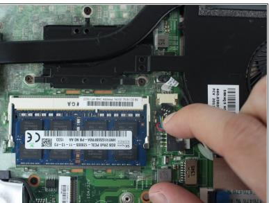
Unplug the Fan connector from its socket on the motherboard.
