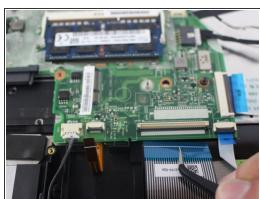
• Lift the beige latch of the ribbon cable with the blue tab by holding the cable in to the motherboard, and with a pair of tweezers, pull out the cable.
