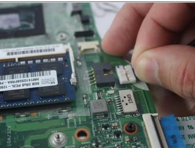
Unplug the remaining connector besides the RAM module and remove it from the motherboard.
