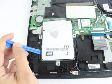
Slide the drive away from the connector by applying pressure on the two side tabs where screws were removed. Use a plastic opening tool as a lever to lift the drive out.
