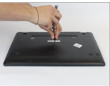
Using the Phillips #0 screwdriver, remove the (11) eleven 5.4 mm screws from the back panel.
