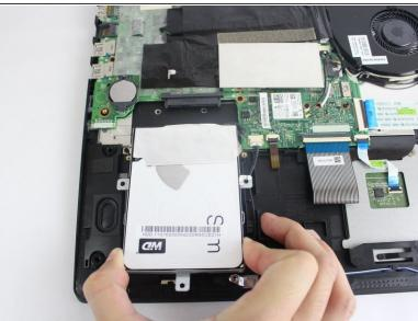
Carefully, using your hand, remove the hard drive from the laptop.
