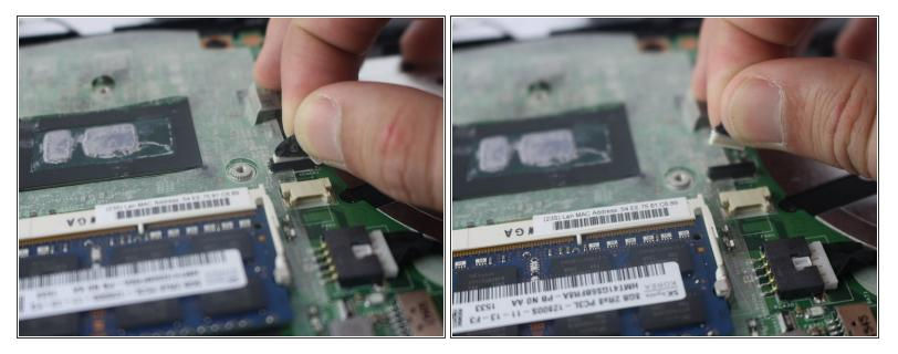
Grab the small black connector by the RAM module and disconnect it from the motherboard.
