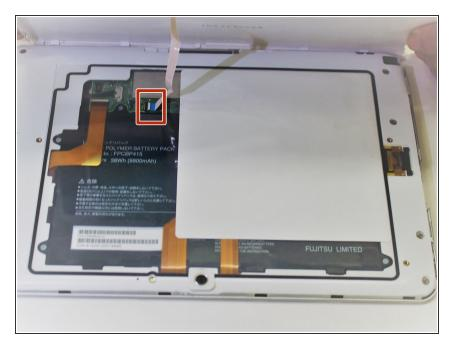
Carefully lift the back case and remove the smartcard ribbon from the motherboard.
