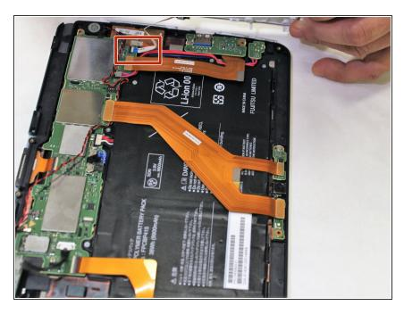
• Lift the shield away from the device and remove the fingerprint scanner's ribbon from the motherboard.
