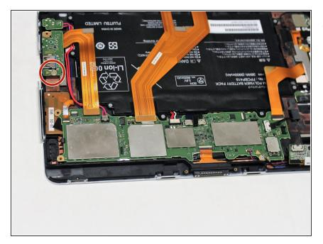
Remove 2mm screw with a PH1 screwdriver from USB board
