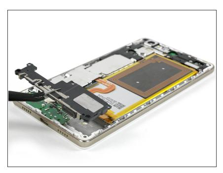
Remove the loudspeaker carefully.
