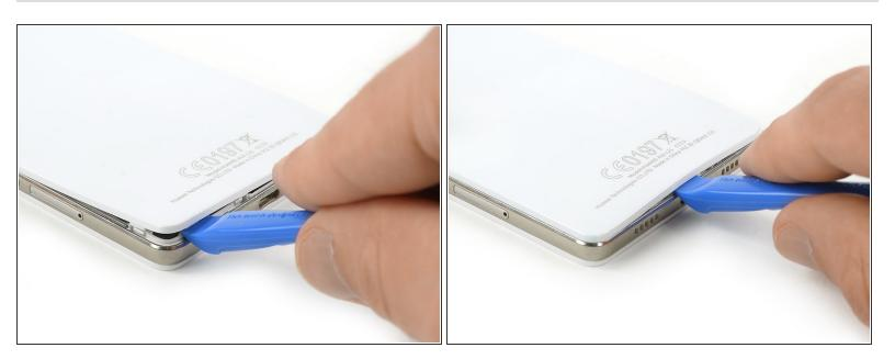
Use an Opening Tool and start to lever up the back cover of your Huawei P8 Lite at the bottom of your phone.
